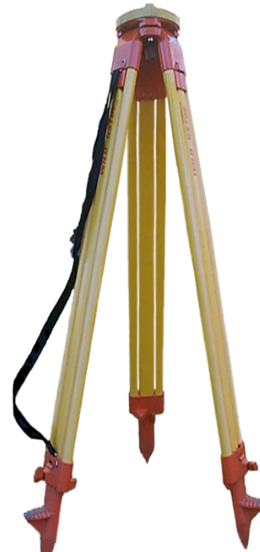
Tripod with optical or physical plummet
